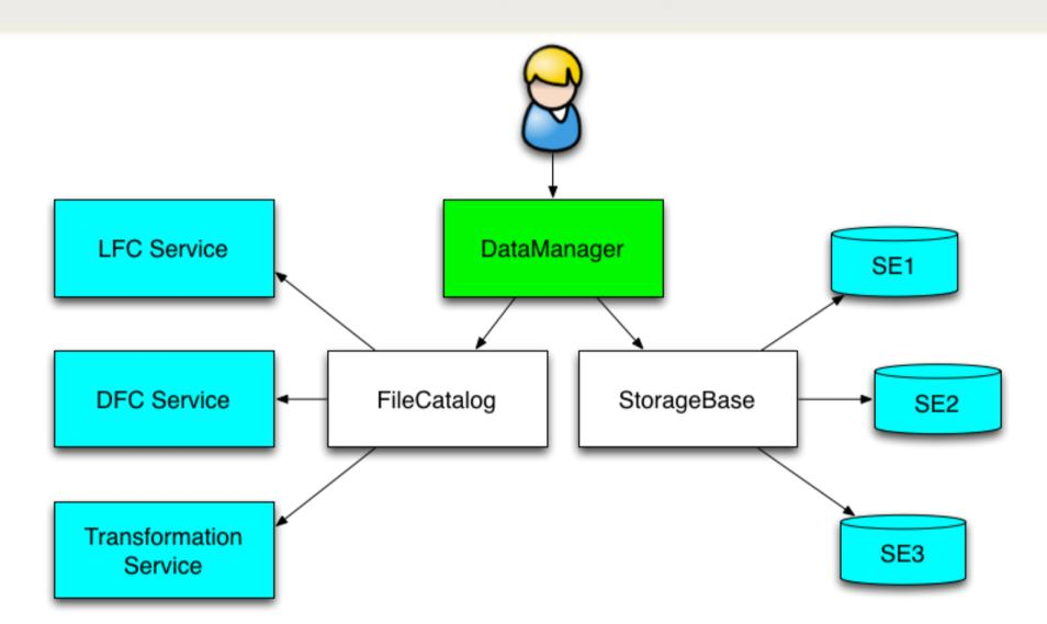
**DIRAC Data Management System** is based on the abstraction of Storage *Elements* and *File Catalogs*. This allows to present all the distributed user data as stored in a single logical file system.
